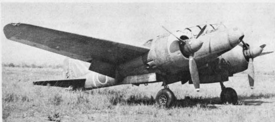
Dinah 3 , the latest version of this standard Jap recon plane, has a new nose. A rounded and
